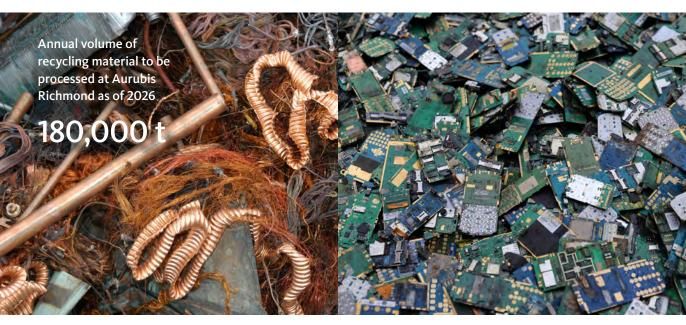
A variety of recycling material input: shredder materials, copper wire, and printed circuit boards (PCBs).
