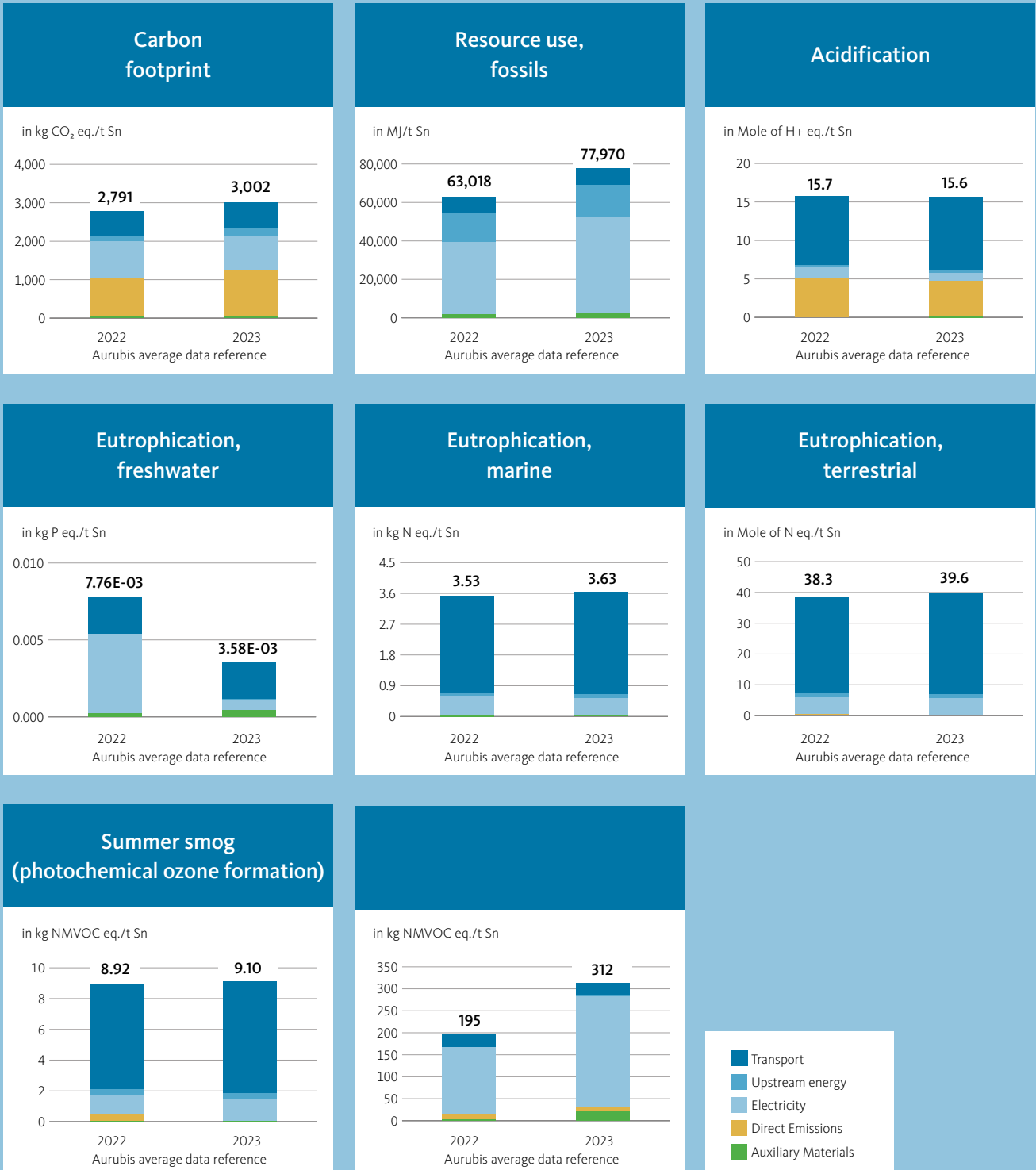
Figure 1: Results for 1 ton of Aurubis Beerse Tin ingot (2022) and (2023), (Environmental footprint EF 3.0)
