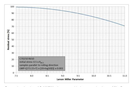
Stress relaxation data of CuNi3SiMg shown as residual stress against Larson Miller Parameter. The Larson Miller Parameter represents temperature and time. Test method: Mandrel test according to ASTM E328.
